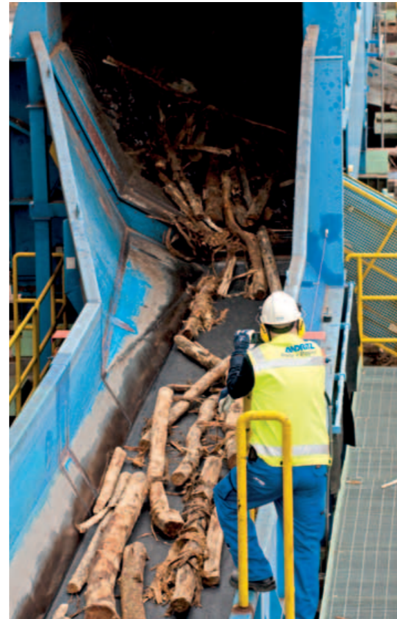
▲ Ilkka Manninen, ANDRITZ Sales Manager for wood processing systems, at the RotaBarker. The efficient separation of bark eliminates the roping effect of Acacia bark which typically occurs with conventional drum debarking lines.
