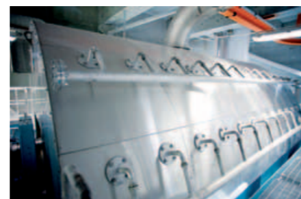
▲ A view of the LimeDry filter for drying lime mud prior to burning in the kiln. ANDRITZ also delivered a LimeWhite filter to enable the mill to meet future targets for white liquor production.
