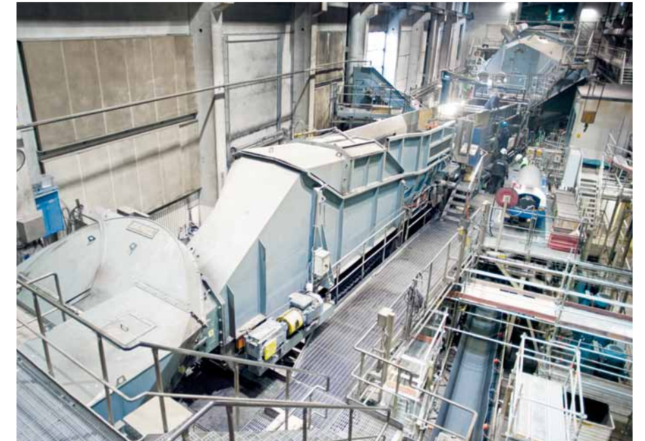
▲ ANDRITZ HHQ-Chipper installed at the Gävle Mill. “A remarkable piece of technology,” according to Thomas Björklund
