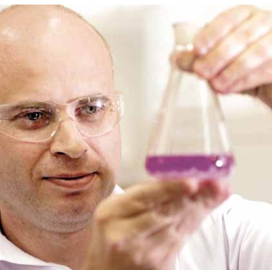
▲ Piracicaba's Pulping Lab Analyst, Marcelo Tognim, performs a lab test for ash content. Manual laboratory inputs are used by the control strategy developed by the OPP service to predict the mineral load and automatically compensate for it when an operator changes production rates or alters the ash-to-fiber ratio.
