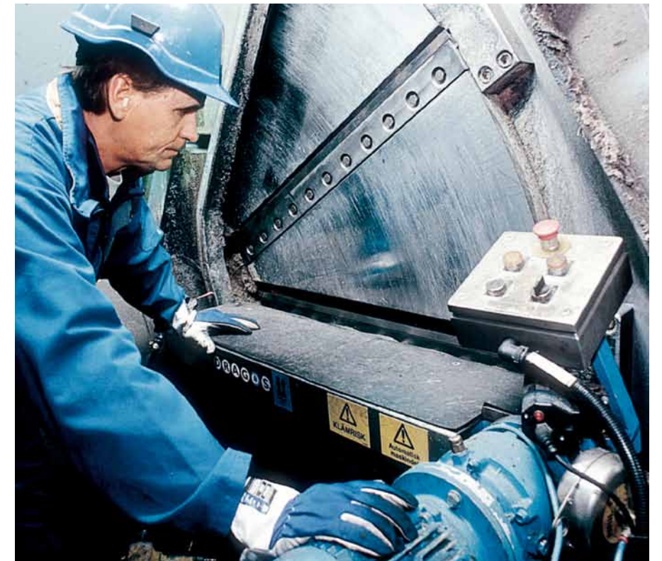
▲ Maintenance person inspecting the TurnKnife system – an easily manageable knife system with two edges – that produces the highest quality chips over the longest time.
