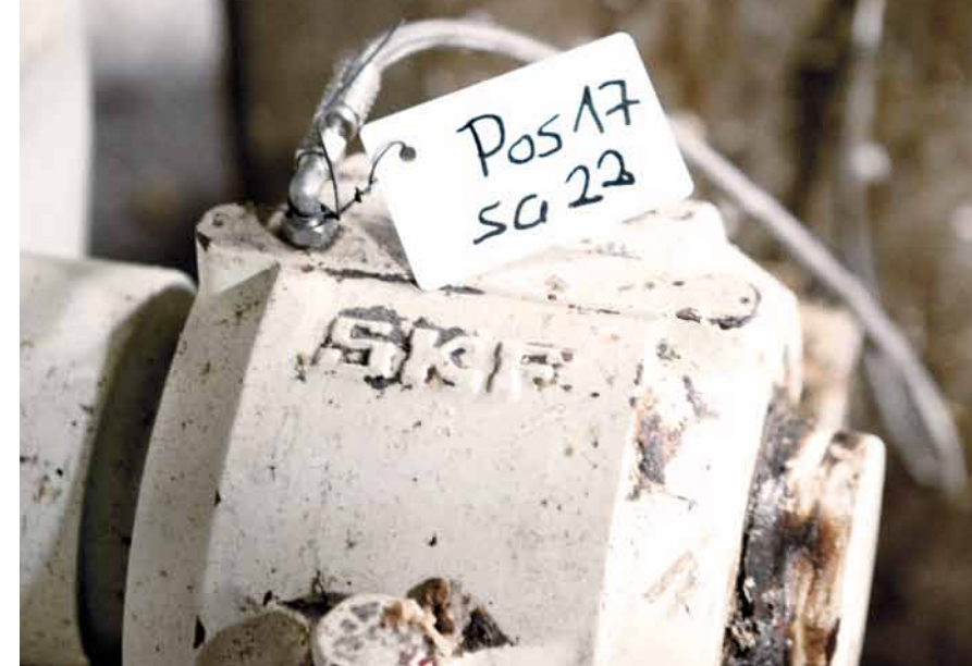
▲ Each piece of the dismantled machine is inspected, condition noted, and tagged before being placed in one of 250+ containers for shipment to Russia.
