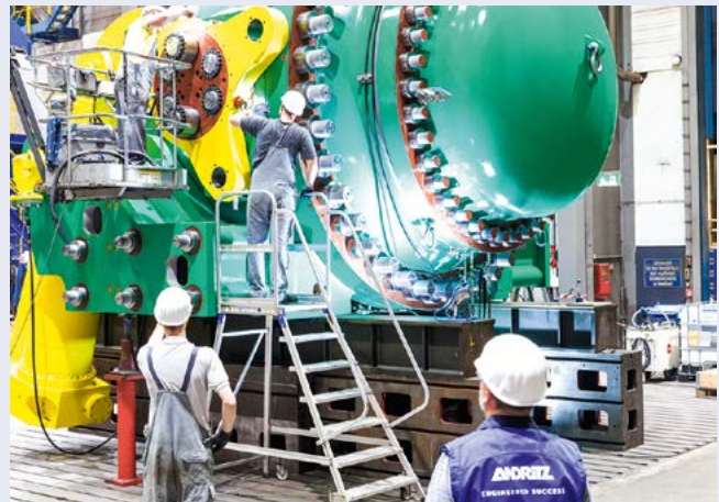
Pressure test and Factory Acceptance of the first of six spherical valves for Dinorwig in the presence of the customer in autumn 2022
