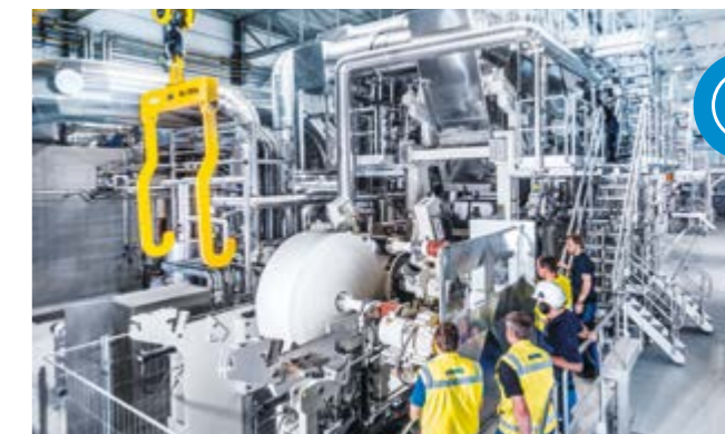
The ANDRITZ tissue pilot plant in Graz, Austria – the PrimeLineTIAC – is currently configured as a PrimeLineTEX machine and offers customers the opportunity to test and develop their future textured tissue.
