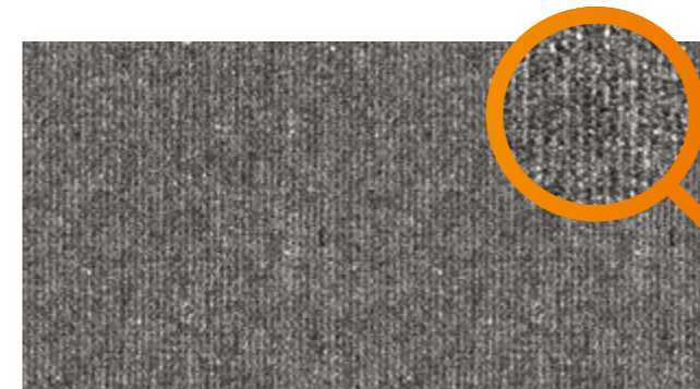
Fig. 7: Conventional fabric design Sample: 15 g/m 2 tissue (pulp + DIP). Speed: 1,750 m/min
