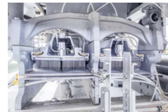
Needlelooms: Pneumatic centralized needleboard pinning system
