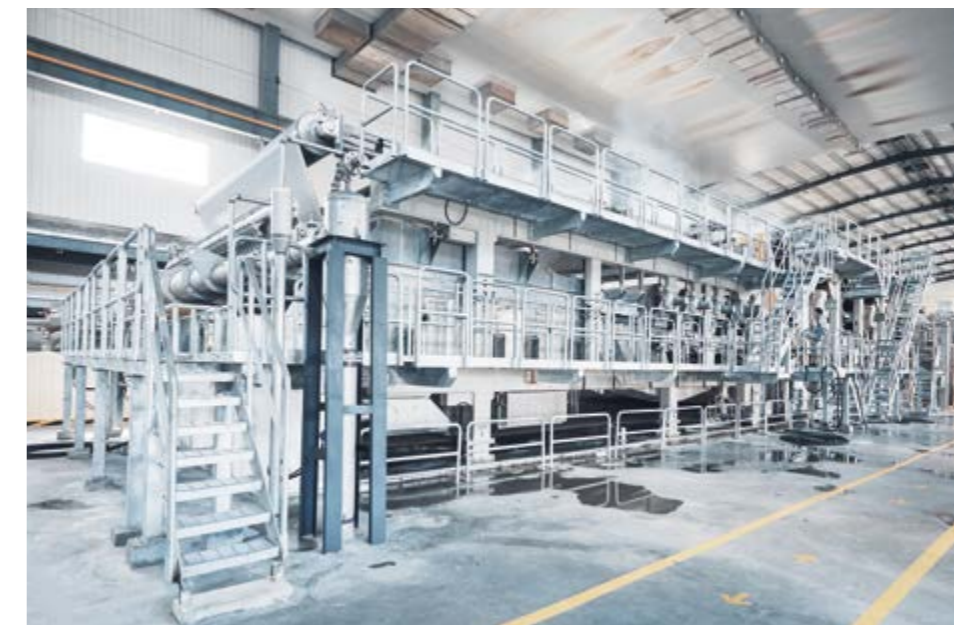
The pulp drying line consists of a TwinWirePress pulp machine, airborne dryer, cutter-layboy, and bale finishing system.
