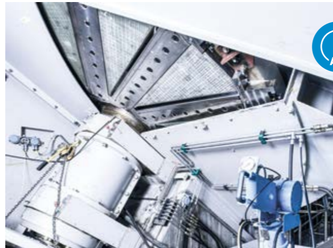
HHQ-Chipper equipped with well-proven TurnKnife TK-IV with QuickClamp hydraulic mechanism to permit very fast and safe knife changes.
