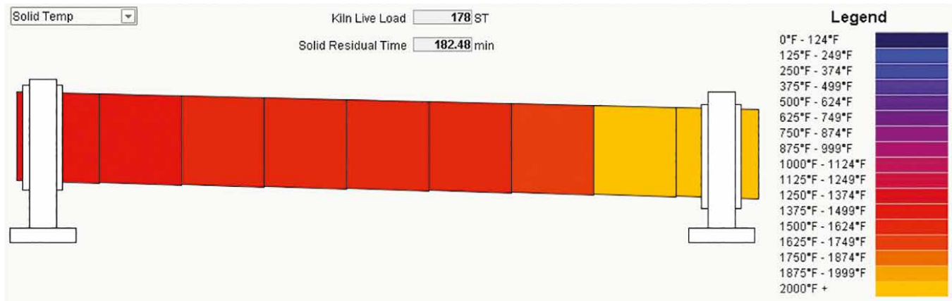
The kiln profiler shows the operator how the temperature varies along the kiln's length.
