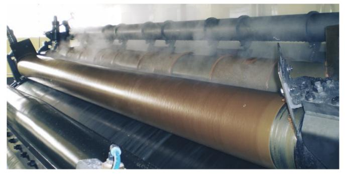
Starch drying on a drum dryer
